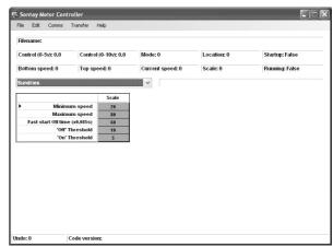
When the input falls below the Off threshold, the output will turn OFF. When the input rises above the On threshold, the output will turn ON.
